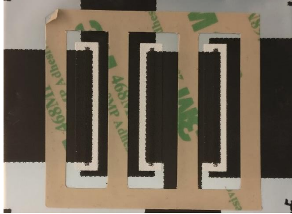
Figure 16. Adhesive tape on monolithic three-cell supercapacitor module.
