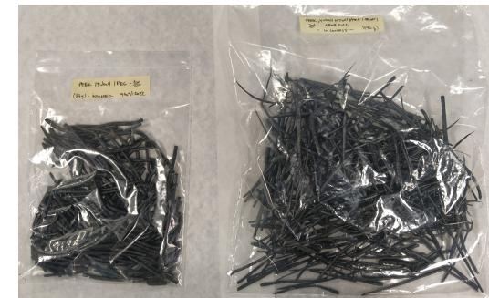
1 st & 2 nd extrusion of PEEK/SWCNTs (2.5 wt%)/PEG (15 wt%)
