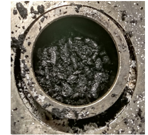
PEEK/SWCNTs (2.5 wt%)/PEG (15 wt%) – 2 nd extrusion step feeding
