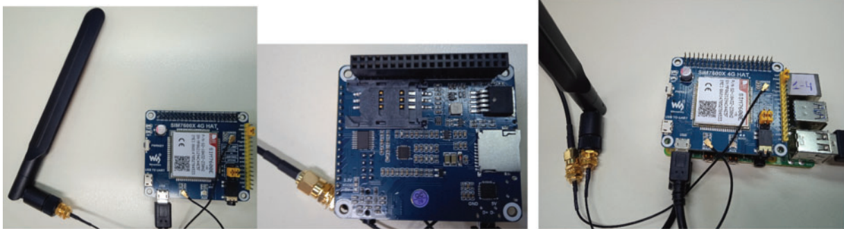
Figure 20: 4G and GPS HAT for Raspberry Pi—Waveshare SIM7600X
