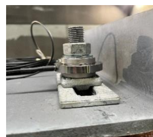
Figure 5. Force washer integration.
